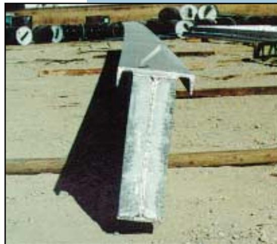
Some fabricated assemblies may distort at the galvanizing temperature as a result of relieving stresses induced during manufacturing of the steel and in subsequent fabricating operations
