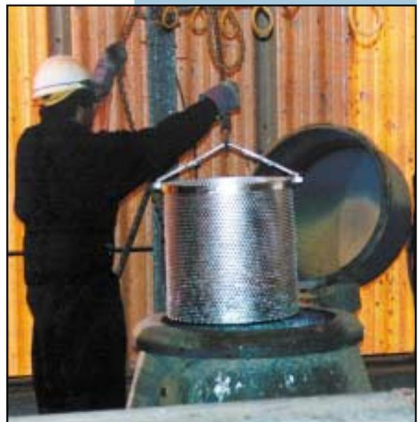
A perforated basket filled with bolts is placed in a centrifuge to spin off excess zinc
