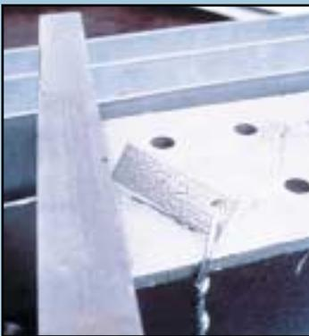
A deep stenciled steel tag firmly affixed to the fabrication with a minimum #9 gauge steel wire
