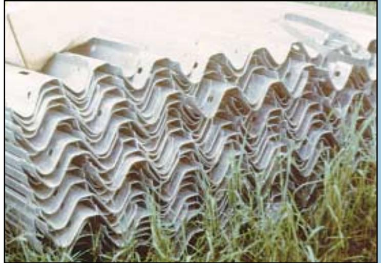
Poor storage, shown here, can lead to wet storage stain
