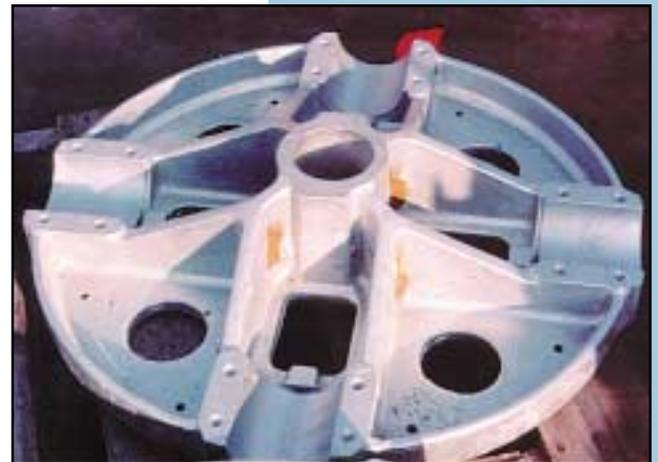
Castings must be abrasively cleaned in order to achieve a fully galvanized coating
