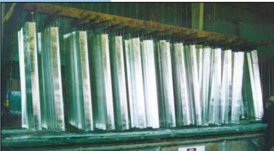
Galvanizers often rack products in order to effectively galvanize more than one product at a time, such as with these guardrail posts, which are being removed from the zinc bath
