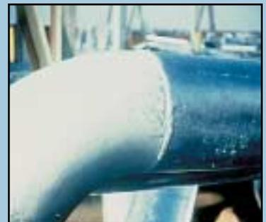
Varying steel chemistries create visually different coatings, as illustrated by this pipe assembly
